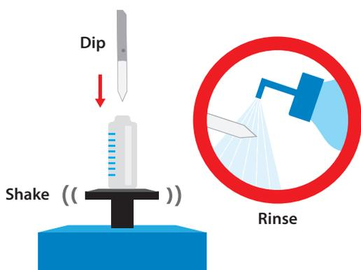
Analytes of interest are collected by the blade's coating. Larger, matrix-related compounds are not incorporated into the coating and are easily rinsed off prior to analysis.
